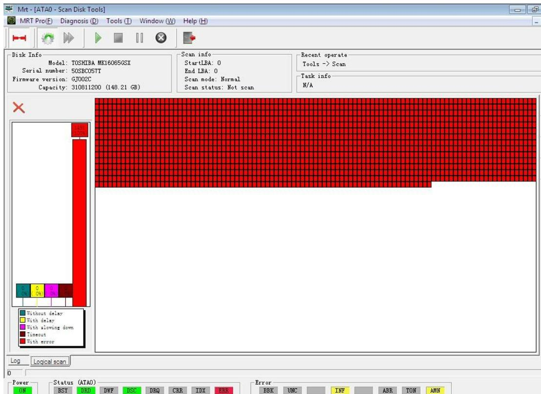
They are all red blocks scanned because when entering factory program, the HDD was switched to Techno On mode in which user sectors cannot be read.
